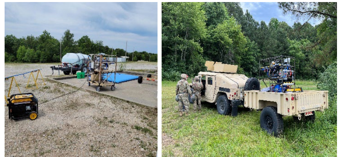
Figure 1. Foreground (left): Final version of the mobile emergency water treatment system cart at the DRIPS Demonstration Ft. Leonard Wood-ERDC CERL Contingency Basing Integration Training, Evaluation Center (CBITEC) Demonstration 2023; (right) FT Barfoot 2024 Quartermaster Liquid Logistics Exercise (QLLEX). Deployable Resilient Installation water Purification and treatment System (DRIPS).
